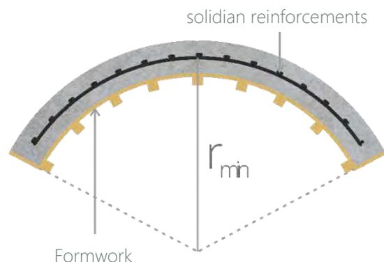
Figure 12: Installation only in compliance with the minimum permissible radius of curvature
