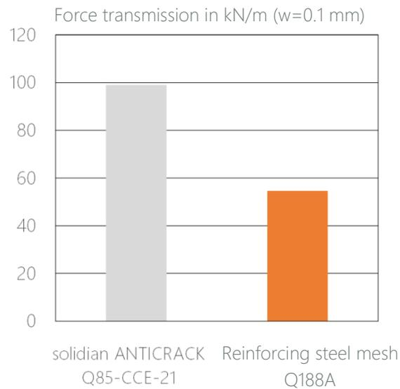
Figure 22: Exemplary comparison of the force transmission of solidian ANTICRACK and a reinforcing steel mesh in a rising crack with a crack opening of 0.1 mm
