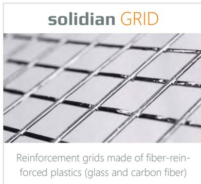
solidian GRID is a bidirectional reinforcement grid made of media-resistant carbon or glass fiber composite plastic. It is preferably used in load-bearing, flat concrete components to absorb tensile forces. solidian GRID is characterized by its corrosion resistance, which reduces maintenance and replacement costs in the long term. It also offers maximum design freedom, so that even the most demanding architectural visions can be realized without compromising on material strength or durability.
