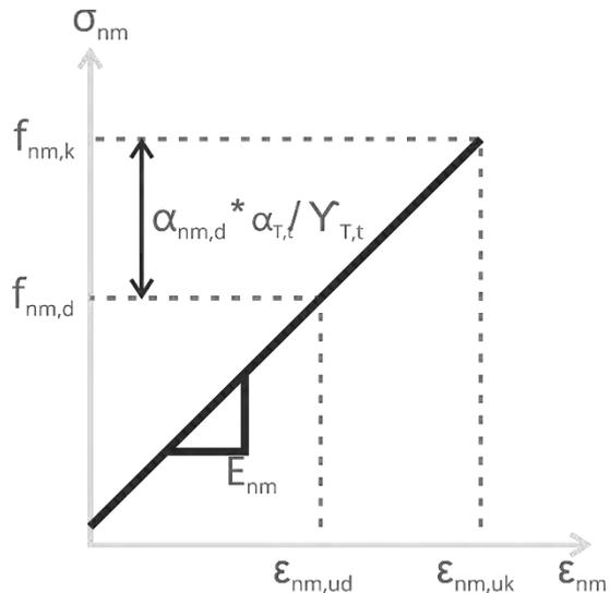
Figure 21: Calculated stress-strain curve of the non-metallic reinforcement for the design for tension
