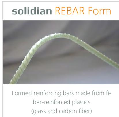
solidian REBAR Form is a shaped reinforcing bar made of media-resistant carbon or glass fiber composite plastic. These durable reinforcing bars are used in structural and statically relevant concrete constructions, especially for absorbing tensile and shear forces. solidian REBAR Form is formed in the factory and delivered to the construction site ready for installation.
