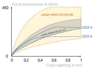
Figure 24: Force transmission of the reinforcement in the opening crack - comparison of typical reinforcing steel meshes with glass and carbon bars
