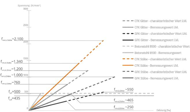
Figure 3: Stress-strain relationships in comparison
