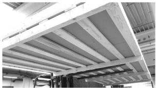
Figure 9: Pallet transport for flat reinforcement grids
