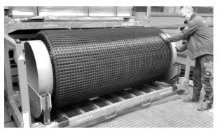
*Figure 6: solidian CARGO System stacking and transport rack with unwinding device*
